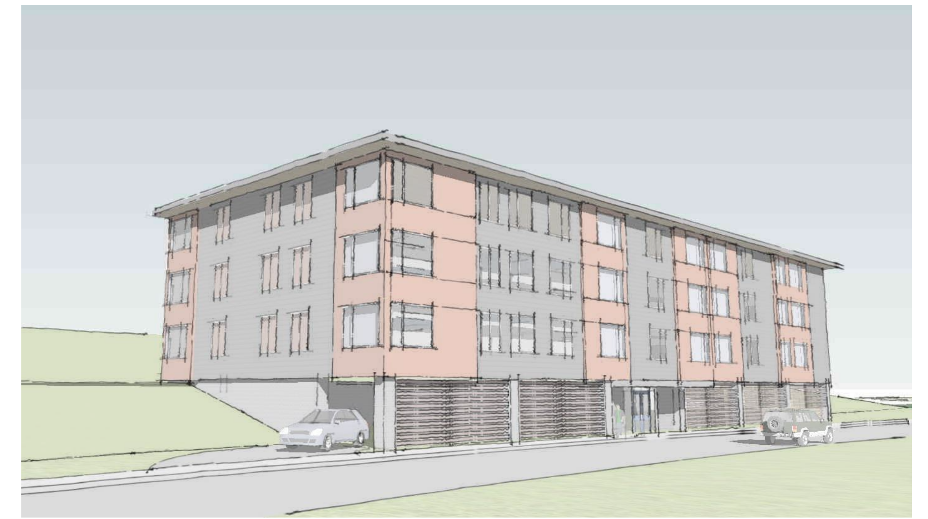
Sloped Site Design Concept: parking under building
